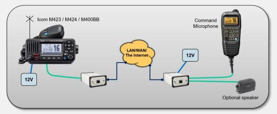
Example of set up with Icom IC-M423 and Command Microphone
