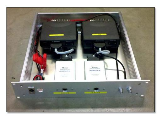
In this example with two Tetra radios and two Network Interfaces in each rack unit.
