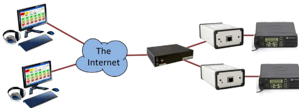
*Typical setup where a RadioServer is needed, with two radios and two remote operators*
