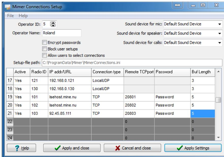
*Example of Mimer Connection Setup, in an Operator PC.*
